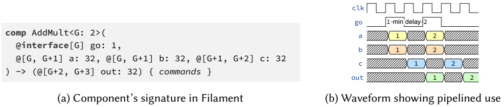
Fig. 4. Signature and waveform diagram. The component allows pipelined execution or reuse after two cycles allowing overlapped execution. Shaded regions represent unknown values.
